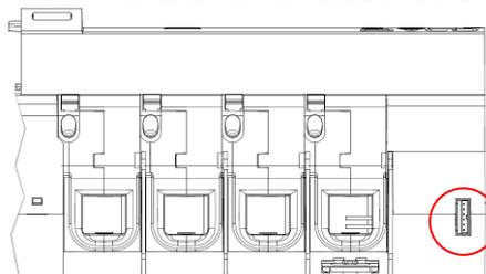
The port enables the integration of the device in the monitoring system via the RS485 communication interface (ref 4 210 75) and the Gateway RS485/IP.
