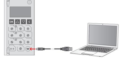
In order to use Power Control Station software the electronic device has to be connected to the PC
