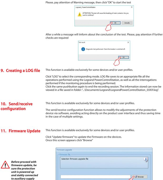
*module.* An incorrect or instable supply can interrupt the updating process and corrupt the device firmware, compromising its correct working.
