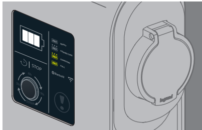
"Borne sous tension" (blanc fixe) "Charging station energized" (steady white)
