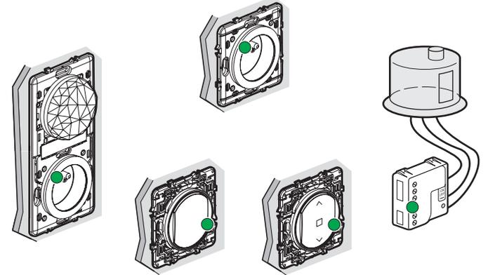
**2 Pair the wireless, batteryless switch to control the connected products (switch, micromodule, socket-outlet, latching relay).**
