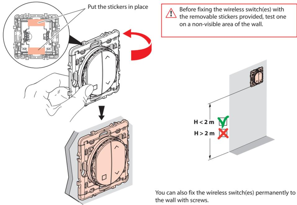
You can also fix the wireless switch(es) permanently to the wall with screws.
