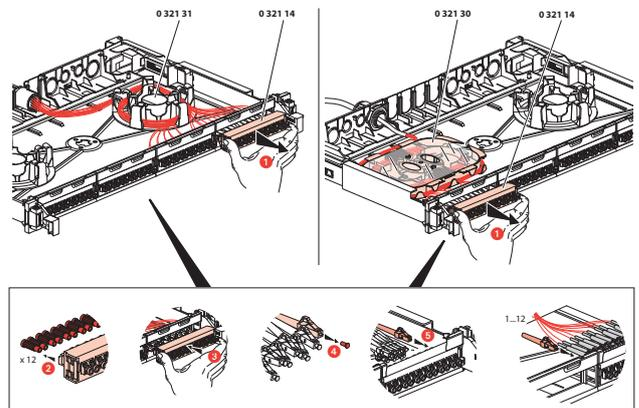
5. BLOCS FIBRE OPTIQUE
