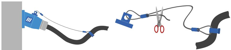
The tension cord has a loop at one end and a cable tie, for clamping the power cable or at a fixed point. A crimping lug allows looping the other end, once passed through to the releasing device and cut to the desired length.
