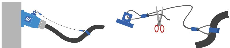
EYELET : Some handles are equipped with an eyelet. This eyelet allows an optimal pulling angle of the tension cord on the latch release mechanism.
