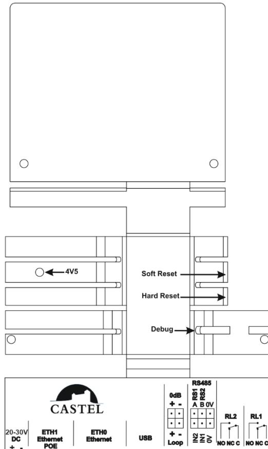
**Connection to the VDIP RS485 bus *Configurable with CASTELSuite***
