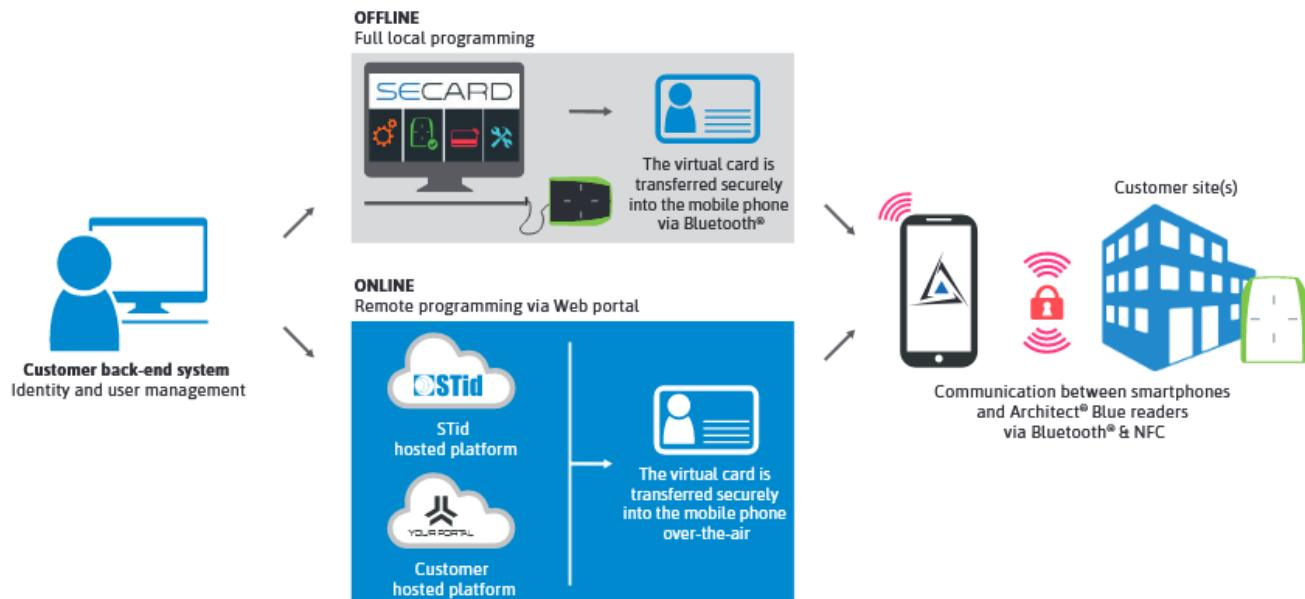
The secure and user-friendly identification solution STid Mobile ID® transfers the access badge to Android™ and iOS® smartphones, in addition to or replacement of the traditional RFID card.
