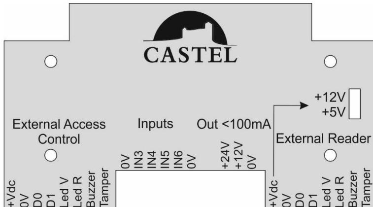
**Connection of external access control system (External Access Control)**
