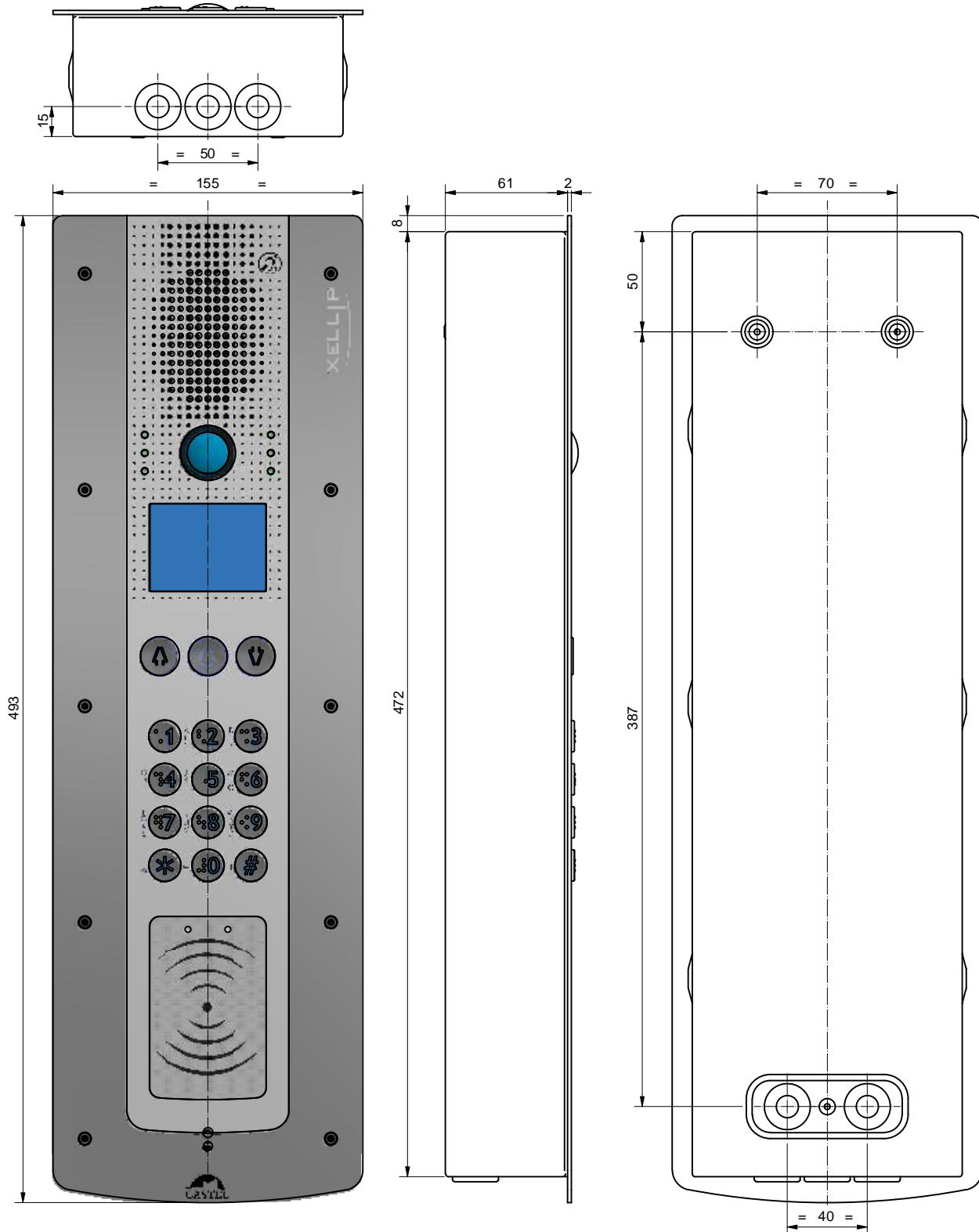
**Surface mounting of models with numeric keypad**
