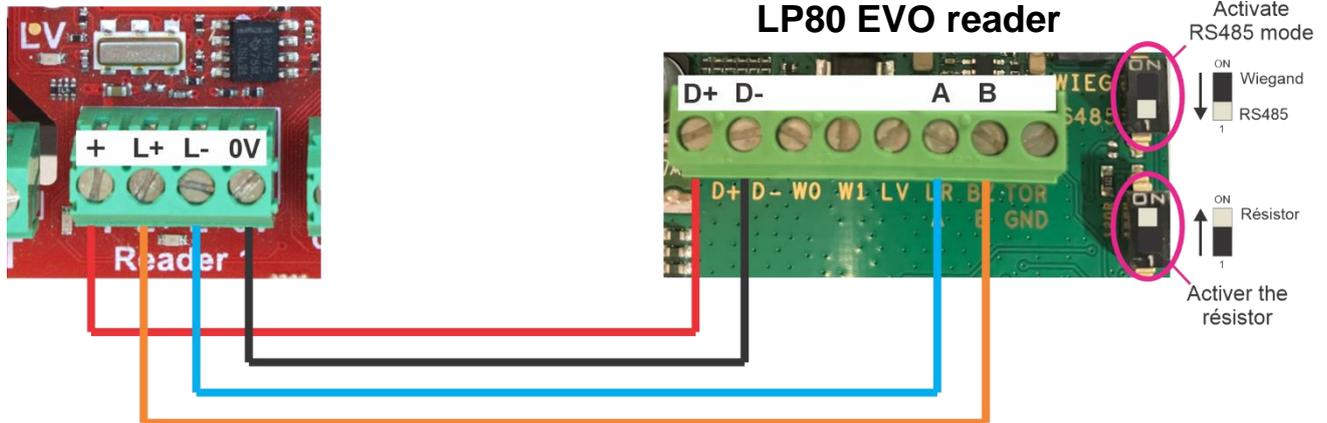
Maximum distance between the reader and the UTP - OSDP: 100m in 9/10 or 0.22mm<sup>2</sup>.
