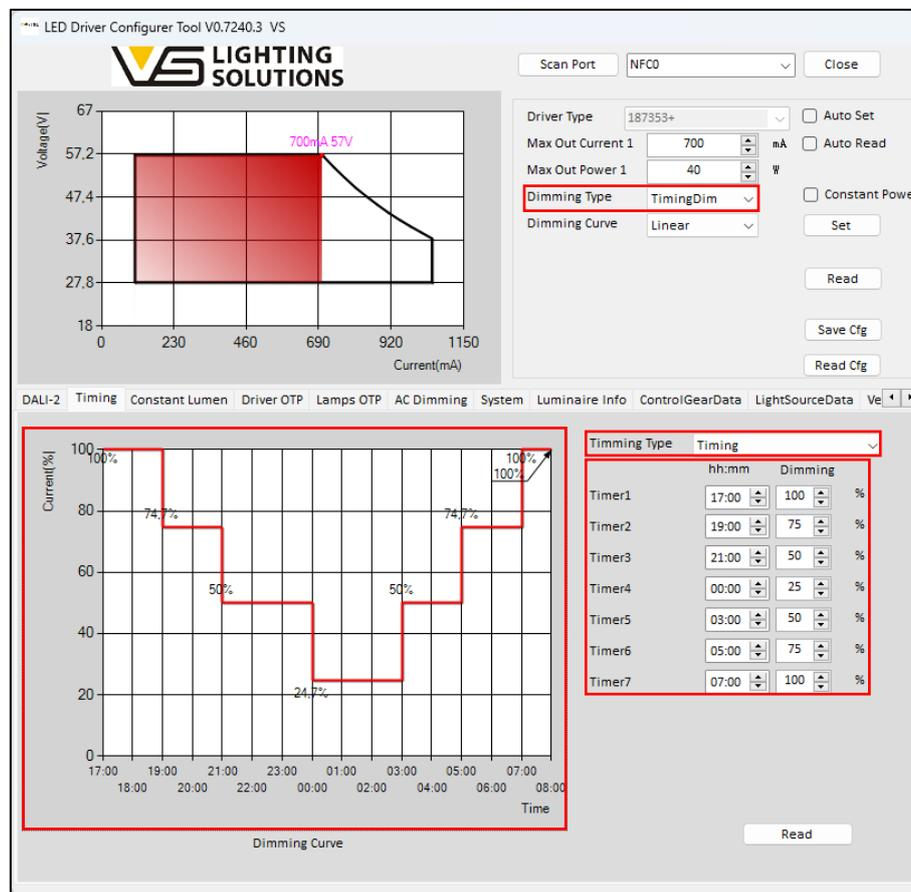
Image 24 – Timing dimming - Traditional timing
