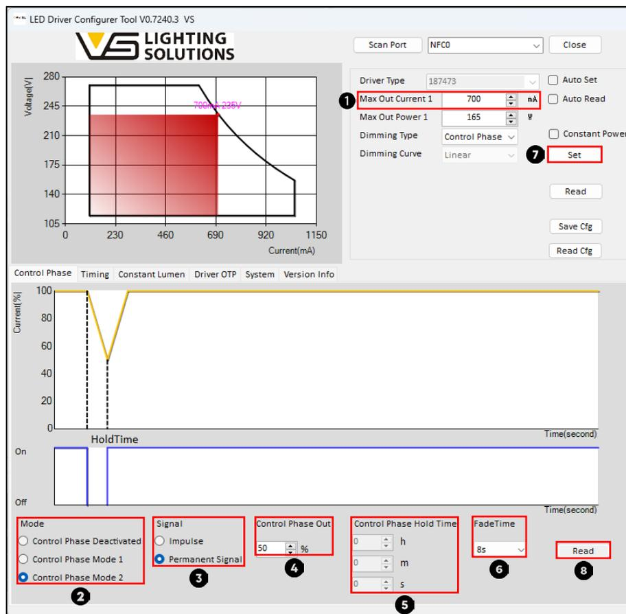
Image 41 – Control Phase Mode 2 – Permanent signal
