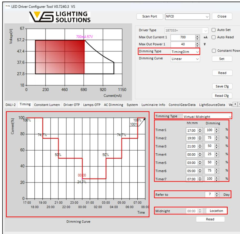
**Image 25 – Timing dimming - Midnight function**
