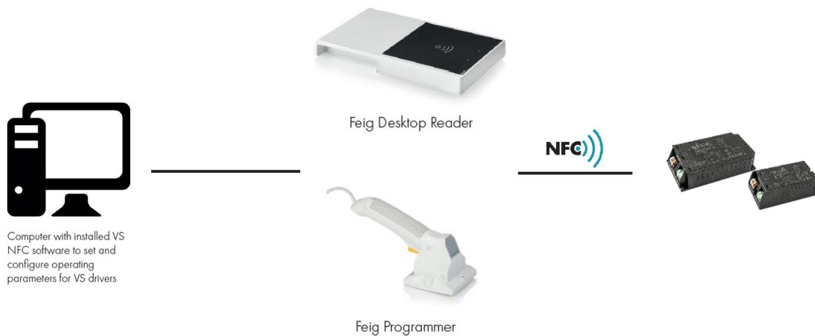
**Note:** For the configuration of LED drivers via NFC, the LED driver must not be powered on. Please make sure that the NFC programming device is close to the NFC interface of the LED driver (check exact antenna position on the driver label) - the distance must be  $\leq 30$  mm.
