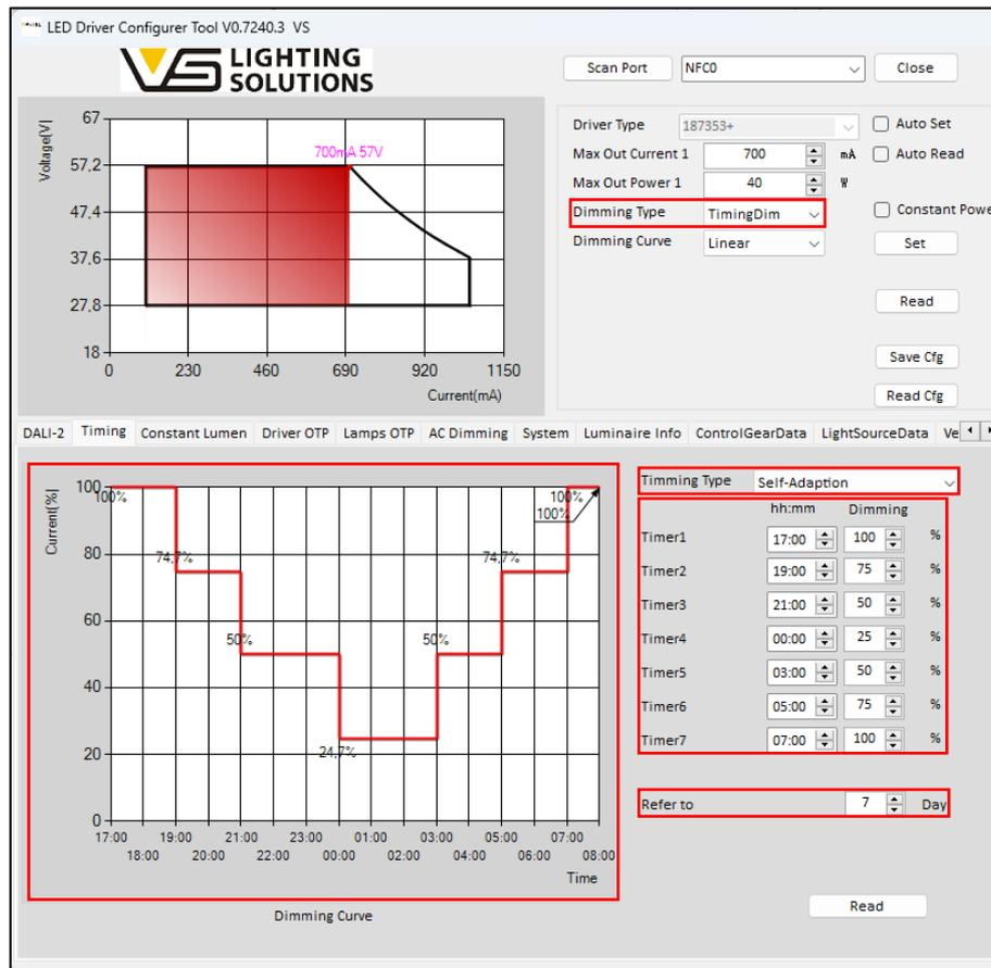
**Image 30 – Timing dimming - Self-adapting Midnight**
