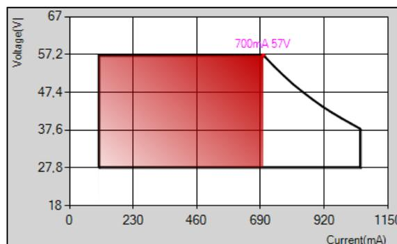
Image 18 – Output window (current vs. Load)
