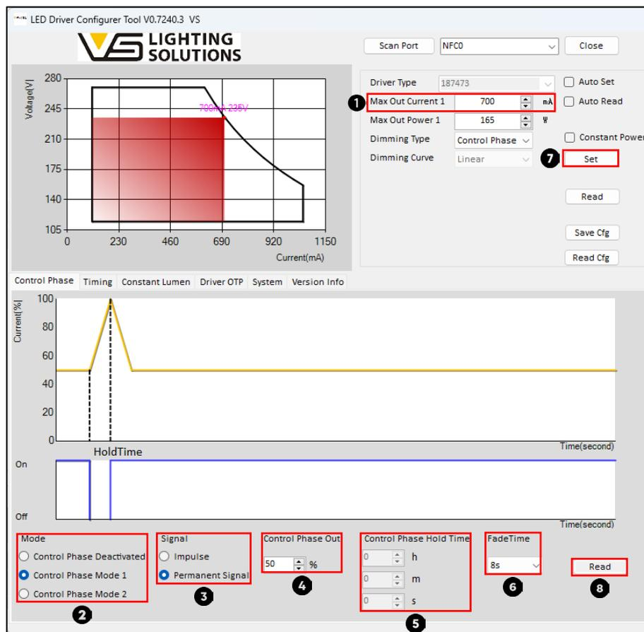
Image 39 – Control Phase Mode 1 - Permanent signal
