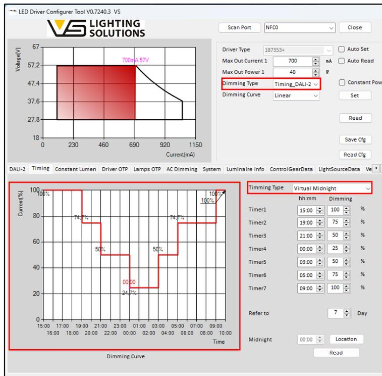
Image 31 – Timing dimming DALI2 - Midnight function
