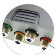
LNB Quattro Convertisseur universel VB > Vertical Bas = 13V - VH > Vertical Haut = 13V+22KHz HB > Horizontal Bas = 18V - HH > Horizontal Haut = 18V+22KHz
