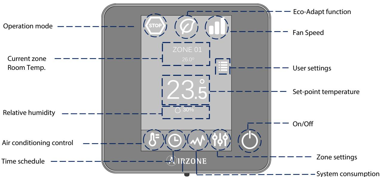
**Operation modes.** Select among the available modes: heating, ventilation and stop. (*See section air conditioning control and operation modes*).
