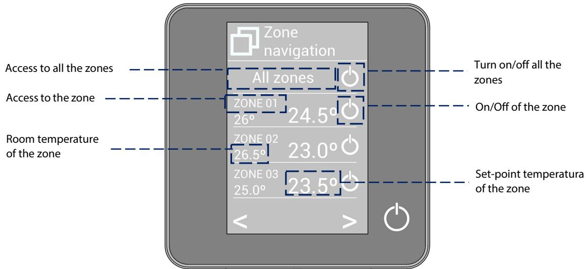
The "All zones" option gives access to the control of all the zones at the same time, broadcasting the changes to all of them. Press on the zone's name to access to all the parameters of the zone and control them from your controller. When the system detects a temperature error on a specific zone, the zone displays the error code instead of the room temperature (see section *Warnings and errors*).
