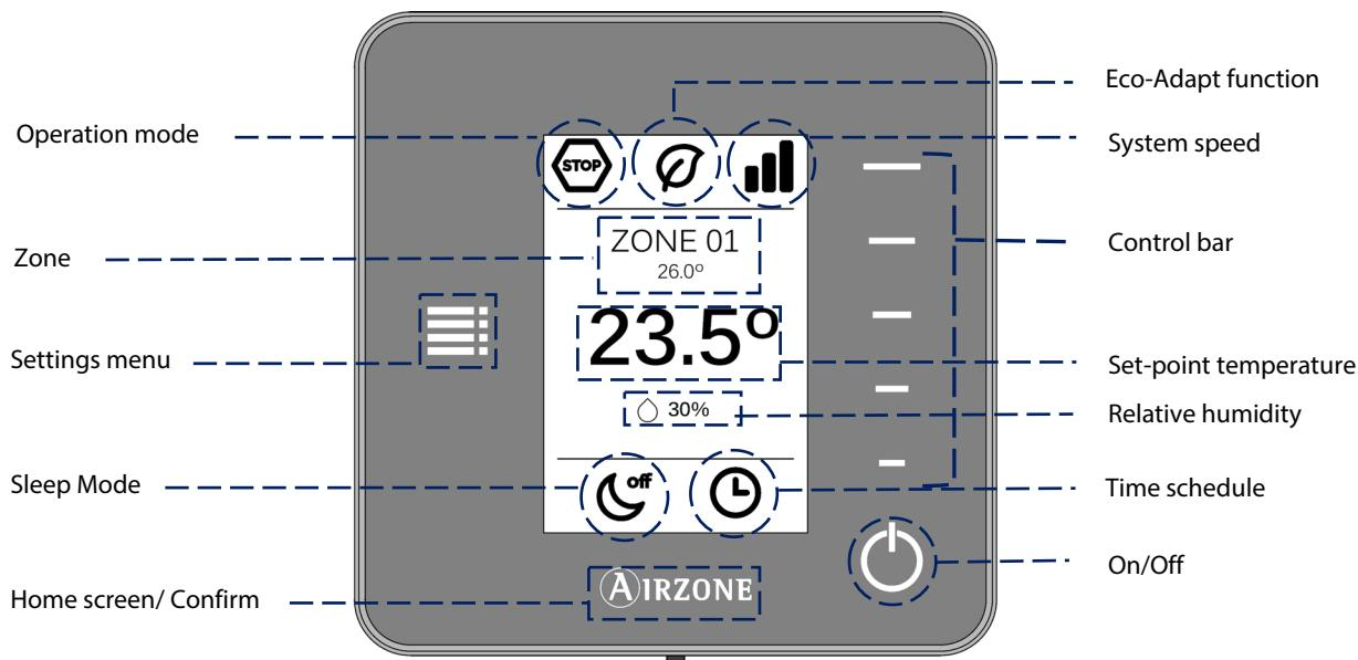
Navigate through the Think Controller by pressing the side buttons on the control bars.
