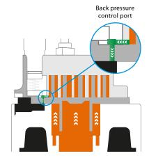
The back pressure control port sends high pressure refrigerant to the back of the scroll ensuring optimum pressure on the scroll.
