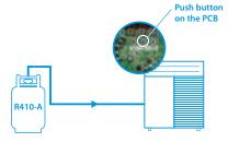
If the temperature drops below 20°C\* manual charging is necessary.
