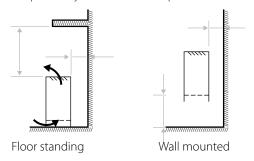
> Wall mounted installation facilitates cleaning beneath the unit where dust tends to accumulate
