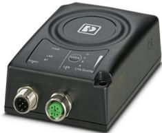
Module radio Bluetooth/Ethernet, 2.1+EDR/4.0, PAN P2P, antenne interne, IP65, 9 V DC ... 30 V DC, raccordement M12, WEB, commandes AT et bouton de mode
