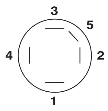
Raccordement QUICKON, 5 pôles
