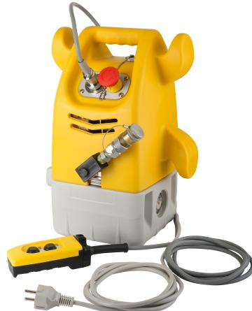
Single acting electrohydraulic pump 220V 50Hz for cutting, crimping and rounding using connectable tools from 50 to 400kN. A 2 ways wire remote control enables full action on this unit (advance, hold and retract). This tool builds pressure and stops when preset pressure is reached. An emergency switch give complete safety over the operation.
