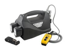
Single acting cordless battery electrohydraulic pump for cutting, crimping and rounding using connectable tools from 50 to 250kN. A 2 ways wire remote control enables full action on this unit (advance, hold and retract). This tool builds pressure and stops when preset pressure is reached. This pump can operate with 1 or 2 batteries.
