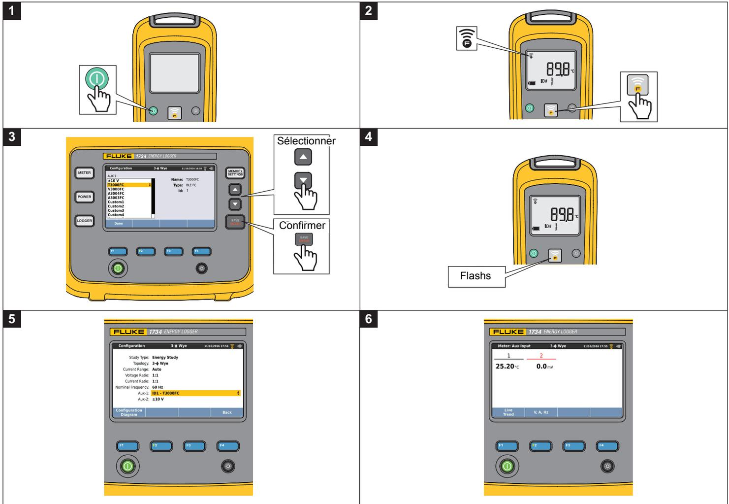
Figure 6. Connexion sans fil aux modules Fluke Connect
