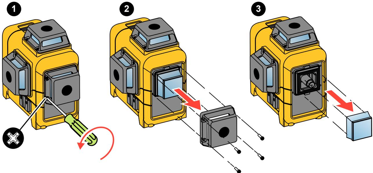
Figure 4. Housing Glass Insert Replacement
