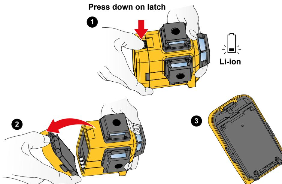
Figure 2. Battery Replacement
