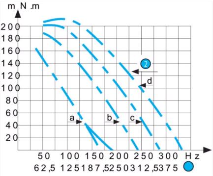
Inertia of measuring chain: 20.5 g.cm2 a = constant voltage controller with Rs (resistance in series) = 0 b = constant voltage controller with Rs (resistance in series) = R motor c = constant voltage controller with Rs (resistance in series) = 3R motor The measurements are made with full stepping, 2-phases energised.
