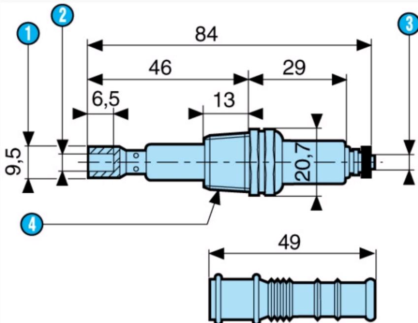
Suitable for high pressures and high temperatures. For use up to 350 °C and 15 kg/cm<sup>2</sup> Metal parts of stainless steel, isolated by ceramic. 3/8" BSP mounting thread.
