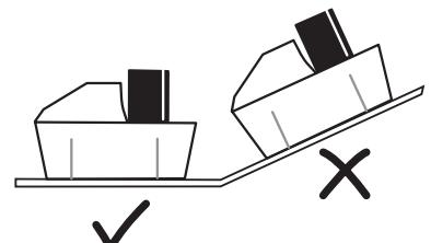
Ensure that there are no kinks or trapped parts in the discharge piping, which must have an internal diameter of 9mm.
