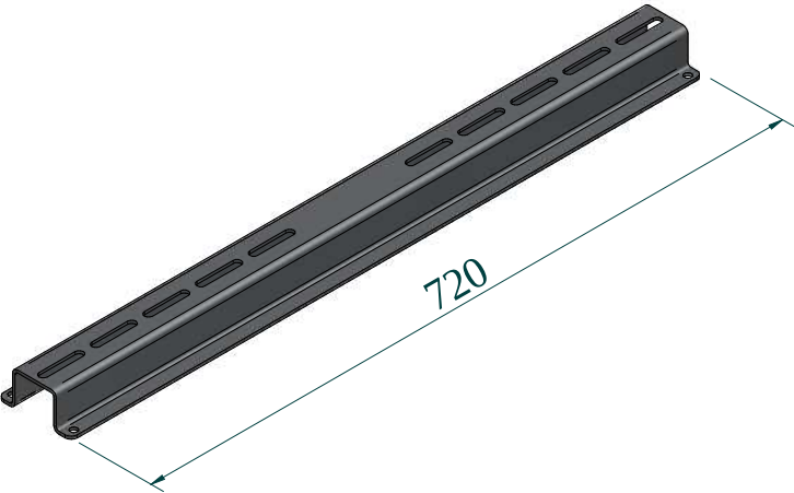
OUTDOOR UNIT BRACKET (Detail)
