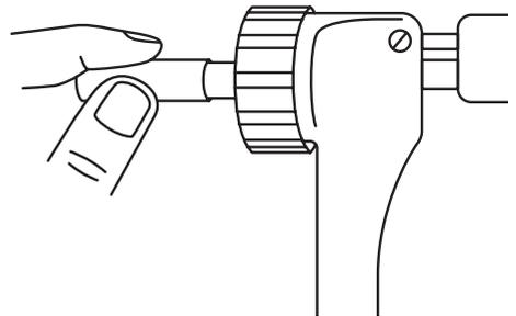
04. Insert the expander head all the way into the tube. **Note:** if the tube opening is too tight, first expand the tip of the tube using the smaller section at the end of the expander head.
