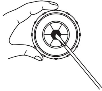
02. Prepare the tube by deburring the inner and outer rims.
