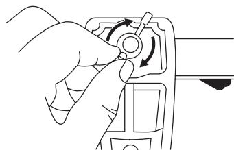
02. Put 'crossbar' on the groove of the bender and lock the wing nut at the bottom of the bender.
