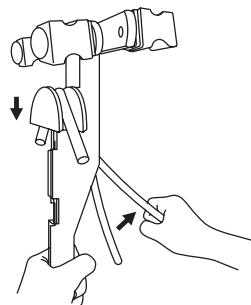
06. Release the lever by pulling it down to allow the 'former segment' to pull back and take tube out.
