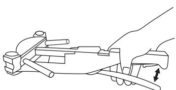
05. Bend the tube to angle needed.
