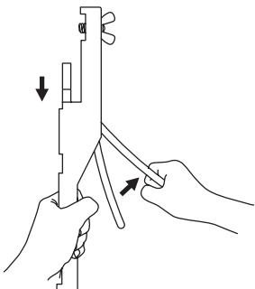
01. Release the lever to let the 'rack' slide to the end.
