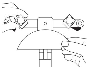
03. Insert your chosen 'former segment' into the rack and turn the sliding piece to the size you want the tube to bend.
