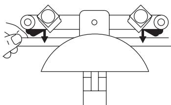
04. Insert the tube into 'former segment', press the lever and let 'rack' move forward to start bending.
