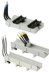
MULTIFIX® 60 is a system for energy distribution comprising a variety of modular combinable components. The energy distribution is carried out via copper bus bars in a 60 mm bus bar system up to 630 A, 400 V AC, 500 V AC, 690 V AC, 45–62 Hz. Short circuit withstand tested to VDE 0660 part 500 and IEC 60439-1.
