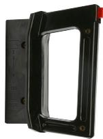
NH- fuse handles are in accordance with the standards of EN 60269 and VDE 0680 part 4/DIN 43620. They are used to insert and remove NH-fuse links and solid links of sizes 00, 0, 1, 2, 3 and 4. These fuse links are in accordance with DIN 43620/1 and are used in NH-fuse bases.
