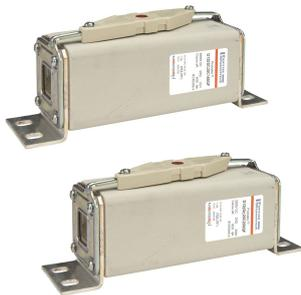
Mersen DC offers provide a very high performant protection for railway power and auxiliary circuits. Mersen DC Semiconductor fuse-links were developed to provide improved performance required by today's new DC equipment. These fuse-links are typically operated at more elevated temperature than other fuse type, have lower  $I^2t$  to minimize damage to protected components on short circuits, lower watts loss and longer life.
