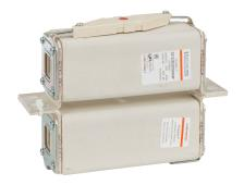
Mersen DC offers provide a very high performant protection for railway power and auxiliary circuits. Mersen DC Semiconductor fuse-links were developed to provide improved performance required by today's new DC equipment. These fuse-links are typically operated at more elevated temperature than other fuse type, have lower I²t to minimize damage to protected components on short circuits, lower watts loss and longer life.
