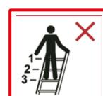
4.33 When the ladder is fully extended, do not climb on the 4th completely reachable rung from the top.
