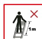
4.34 On a telescopic ladder which is not fully extended, one must not climb or stand on the rungs of the last highest metre.
