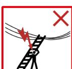
4.26 Watch out for electricity; a ladder is a life-threatening current conductor.
