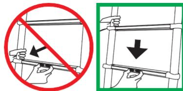
**14** Collapse both top stiles by unlocking both buttons.
