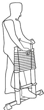
3 Make sure that both top stiles are fully extended and check whether the locking pins automatically click into place. Make sure that there is no red mark next to the buttons.
