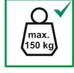
4.11 Never load a telescopic ladder in excess of 150 kg. This includes your own weight, the weight of materials and tool as well as the additional force that arises when working. If you are unsure about the weight, do not use the ladder and consult your dealer or set up scaffolding.
