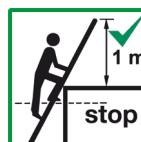
4.16 If you are using the ladder to access a roof, make sure that the ladder projects 1 m above the roof edge so that you have sufficient support when climbing up onto the roof. Do not climb higher than the roof edge to prevent the ladder from tipping over. If not sure, tie the ladder firmly or pin into the ground to secure the ladder base.
