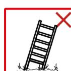
4.22 Place the ladder on a stable surface and make sure that it does not sink into the ground.
