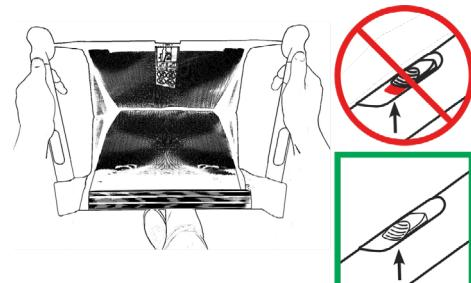
**6** Pull the ladder completely out and check whether each rung is properly locked.
