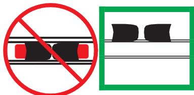
**10** The red lock indicators must be fully visible under the rungs.
