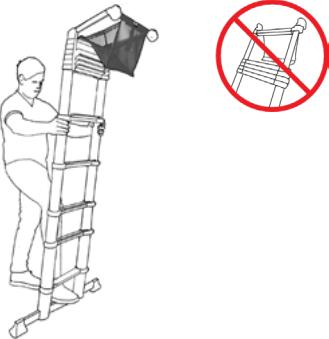
**8** Lean the ladder with the correct slope against the wall. This can be easily checked by placing your feet in front of the ladder and using both horizontally held arms, holding the ladders by the beams.
