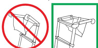
**12** The wall spacer and the tool bag provide you with more comfort and you can lean with your body against the ladder in a better stance.
