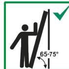
4.13 Place the ladder leaning against the wall with the correct tilt. You can easily check the angle tilt by placing your feet at the ladder's end and extend your arms at a right angle; you should be able to grab the ladder's stiles.
