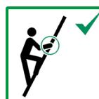
4.15 Keep a secure grip on the ladder when ascending and descending. Maintain a handhold whilst working from a ladder or take additional safety precautions if you cannot.
