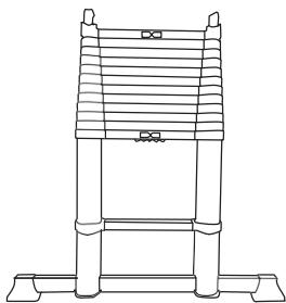
**2** Place one foot on the crossbar to make it easier to pull out the ladder. Make sure that the front of the ladder is facing you, so that the lock buttons are visible.
