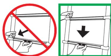
**15** Unlock the arms of the wall spacer by unlocking the lock on the arm of the wall spacer and simultaneously bringing it into a vertical position. Only when both arms are vertical, you can push them back into the ladder stile. Next, fold the tool bag flat and close the Velcro
