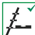
4.17 Leaning ladders with steps shall be used that the steps are in a horizontal position.
