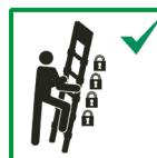
4.14 Check that all rungs are firmly locked and that the green locking indicator is fully visible.
