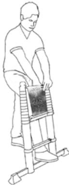
**3** Open the tool bag by opening the Velcro and read the instructions before use. The tool bag is intended for storing small tools and material with a maximum weight of 2.5 kg.
