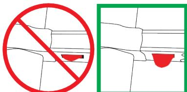
**11** Ensure that the ladder has been correctly positioned against the wall with both rubber wall protectors.
