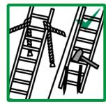
4.9 Ensure that the ladder is secured against slipping at all times. If not sure, tie the ladder firmly or pin into the ground to secure the ladder base.
