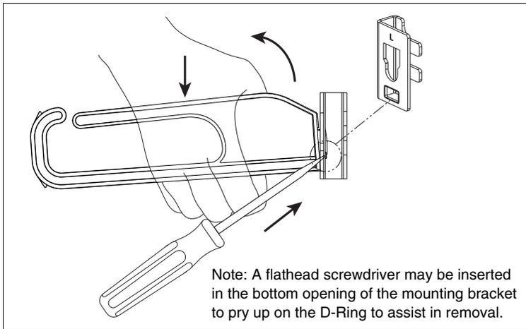
Note: A flathead screwdriver may be inserted in the bottom opening of the mounting bracket to pry up on the D-Ring to assist in removal.
