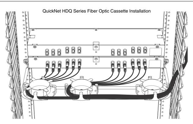
When used with HDQ series cassettes, as shown above, the FQCRCM (shown) can support up to twenty-four MTP\* interconnect cables. The FQCRCM2 can support up to thirty-six\*\*. Only one RU is shown for clarity. Recommended spool positions are shown.
