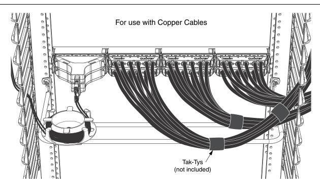
When routing fiber and copper cables in the same RU space, route the fiber separately from the copper cables to avoid damage to the fiber cables. Only two MTP\* interconnect cables (two cassettes) can be supported by the FQCRCM when used with 36 copper cables (6 cassettes).
