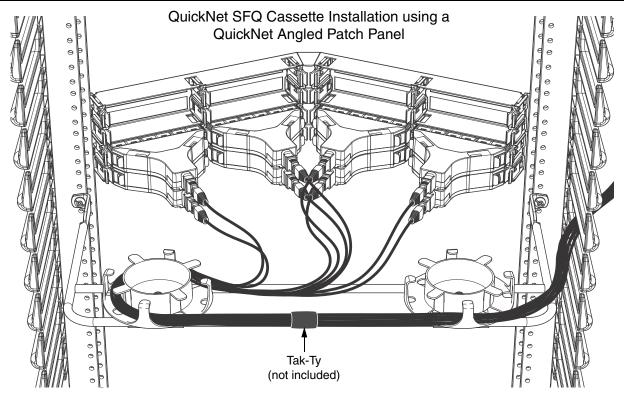
When supporting SFQ cassettes in a QuickNet Angled Patch Panel, interweave the MTP\* interconnect cable for cassettes positioned in the center, as shown.
