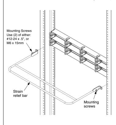
Mount the strain relief bar at the appropriate RU space. Use the lowest screw hole in the RU space.
