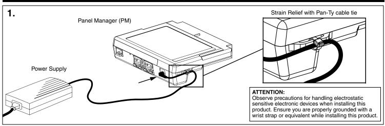
Attach the appropriate end of the AC cord to the power supply. Then insert the power supply's radial plug into the PM. Once the power cord is plugged into the PM, it can be secured to the PM strain relief with a Pan-Ty cable tie, as shown above. Care should be taken when removing the cable tie (if required) so as not to damage the power cord.
