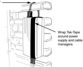
Mount the power supply to vertical cable managers or rack rails on the back side of an installation using Panduit Tak-Tape (Part # TTS-20R0).
