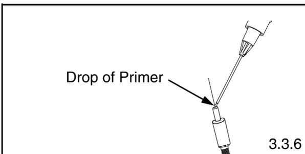
3.3.6 To speed hardening of the adhesive, apply a small drop of primer to the adhesive bead on the ferrule tip using the primer filled syringe. Do not allow the primer to come in contact with the plastic housing of the ferrule assembly. Absorb any primer and unhardened adhesive from the ferrule tip by gently dabbing it with the corner of a lint-free wipe. **Be careful not to break the fiber.**
