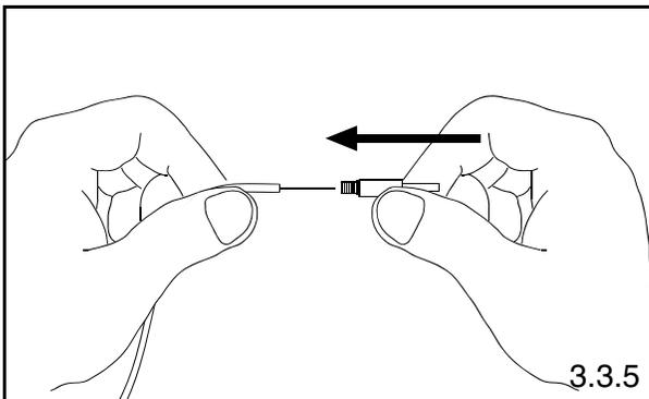
3.3.5 Carefully but quickly insert the bare fiber through the ferrule in a smooth forward motion. The fiber is fully inserted when the buffer bottoms against the rear of the ferrule. The adhesive will begin to set within seconds.
