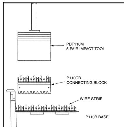
**CABLE REQUIREMENT: Terminates most 22-26 AWG solid or stranded IWC wire with a 0.050" (1.27mm) max. o.d., either PVC or Plenum rated.**
