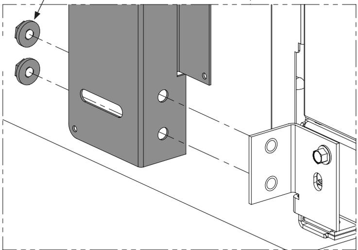
Note the height and side stamping. This stamping is always located at the top and contains a 'R' or 'L' to determine the side of containment, as viewed from the inside of the containment that it will attach to. 'R' for the right side and 'L' for the left side.
