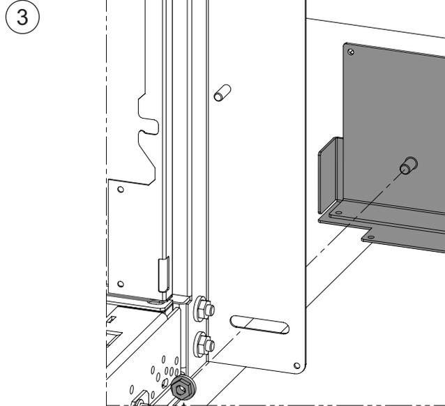
After attaching the Floor Seal. Push the Foam Seal tight against the floor and tighten the 2 M5 x 0.8 Hex Nuts left loose in Step 2.
