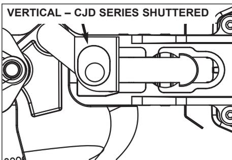
If an older CJD-series shuttered jack module is being used (does not include the newer CJH-series shuttered), the Cam Block Housing Ram oval opening must be rotated to vertical.
