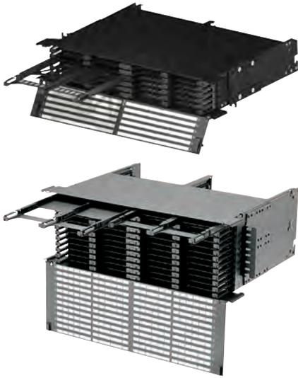
**Enclosures/Panels** – Drawers slide out into locked positions for easy MACs, and house cassettes and FAPs, trunks, connectors, and patch cords. Available in 1-RU, 2-RU, and 4-RU and can be reconfigured to accept 6-port or 12-port, cassettes or adapter panels.
