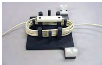
Patch cord compressed into a 2.5-inch coil to form an ellipse cable loop, up to 10 loops total.
