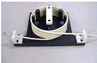
Patch cord put into a 6-inch diameter cable loop, up to 10 loops total.
