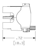
CPCAPBL-X STRAIGHT (HORIZONTAL) WIRE CAP ASSEMBLY FOR FIELD TERMINABLE UTP RJ45 PLUG ASSEMBLY CUSTOMER DRAWING
