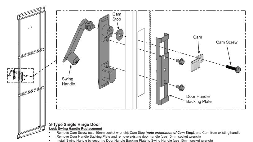
When replacing Cam Stop, ensure that the orientation is the same as when it was removed.
