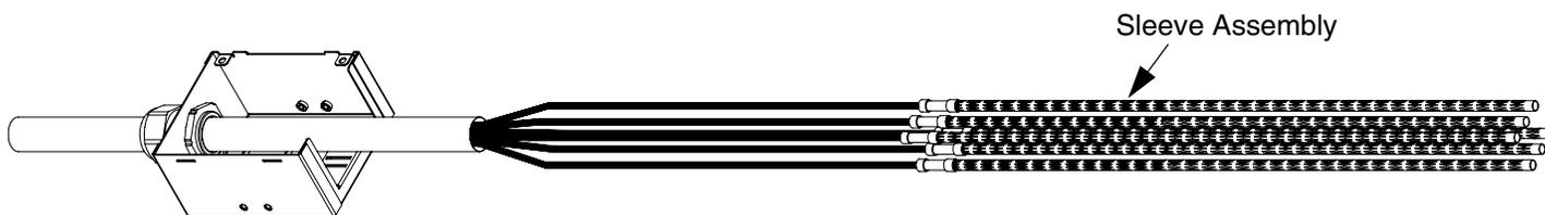
**8. Once the bare fiber is slid fully into the sleeves, snap the sleeves into the transition clip (item 6).**
