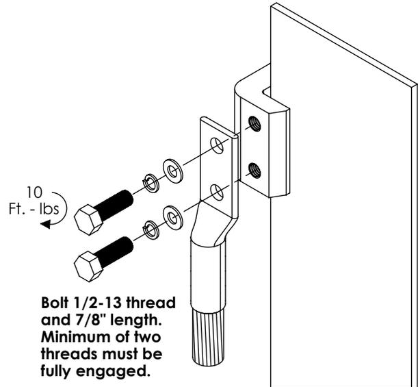
**Bolt 1/2-13 thread and 7/8" length. Minimum of two threads must be fully engaged.**
