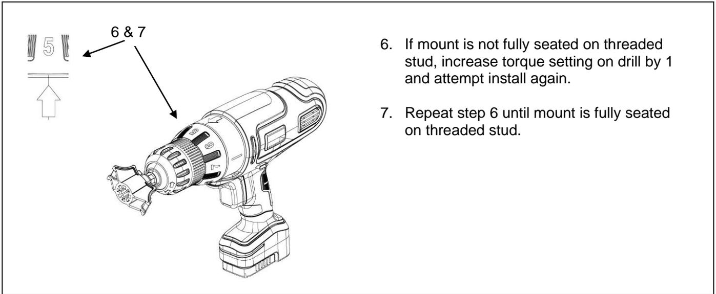
6. If mount is not fully seated on threaded stud, increase torque setting on drill by 1 and attempt install again.
