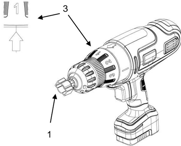
1. Insert TMSTEH-TOOL into 3/8" drill chuck as deep as possible and tighten chuck onto tool.
