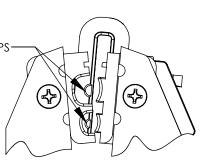
LOCATOR INCLUDES WIRE STOPS FOR PROPER INSERTION OF WIRE INTO CONNECTOR
