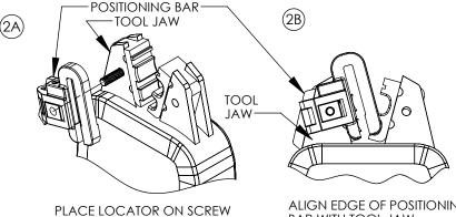
SECURE LOCATOR WITH SUPPLIED LOCKING HEX NUT TO TOOL JAW
