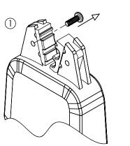
REMOVE SCREW HOLDING UPPER DIE HALF IN TOOL, AND REPLACE IT WITH LONG SCREW SUPPLIED WITH LOCATOR
