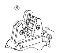
PLACE CONNECTOR IN CRIMP DIE, MATCHING COLOR DOT ON DIE POCKET WITH COLOR OF CONNECTOR INSULATION
