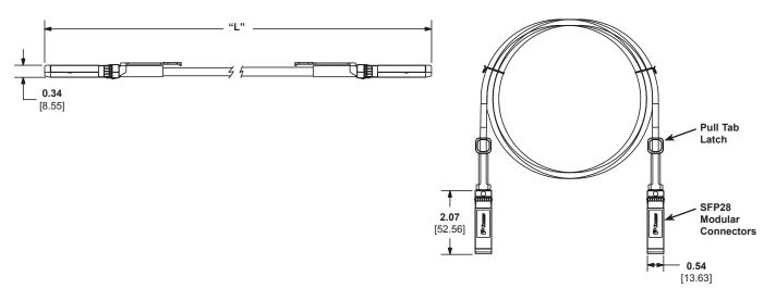
Dimensions are in inches. (Dimensions in parenthesis are metric).
