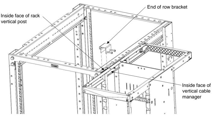
Place end of row bracket around inside face of the rack vertical post and inside face of Vertical Cable Manager as shown.
