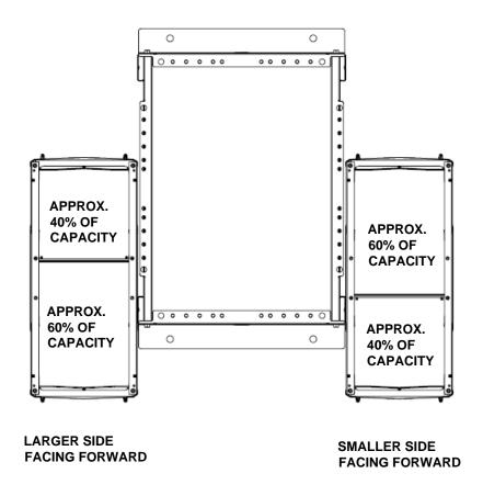
**PATCHRUNNER**<sup>TM</sup> 2 Enhanced Vertical Cable Managers may be installed with either side facing forward.
