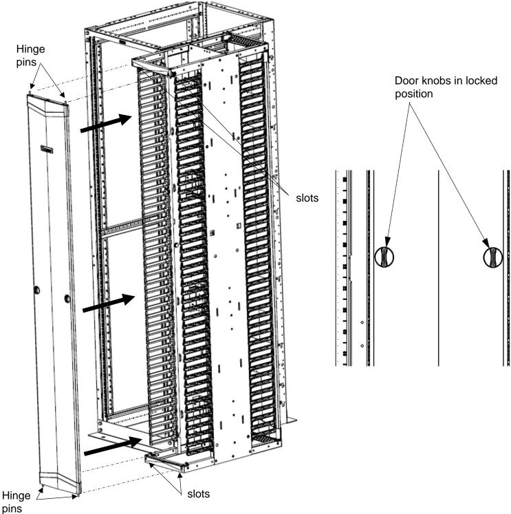
Align Door hinge pins on 4 sides to slots on door supports and simply push closed. The door knobs will be in locked position as shown.
