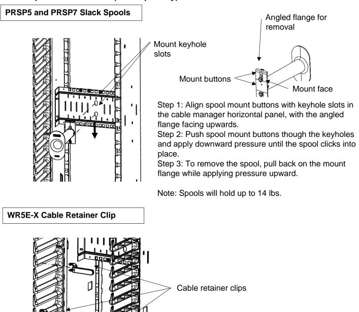
To install cable retainer clips, place the open end of the clip around the leg of the molded finger on the vertical cable manager and position as required.
