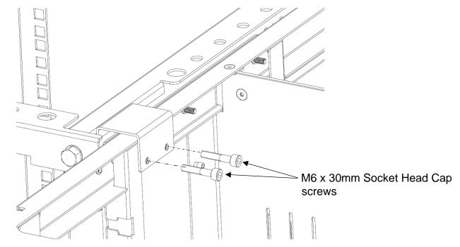
Tighten the end of row bracket using (2) M6 x 30mm Socket Head Cap screws.
