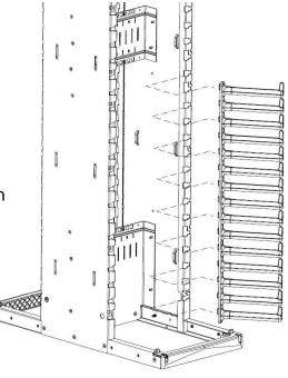
Align finger mount tabs with mounting slots on the manager side panels. Finger sections installed pointed up with the rounded side facing inward. Push toward the outside of the manager until you hear an audible "click". Light tapping with a dead blow hammer may be used to fully seat the fingers.
